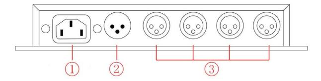
1 AC100-240V power interface 2 DMX signal input interface 3 DMX signal output interface
