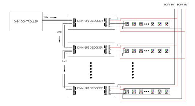
**Double power connect double signal line strip condition:** if the V+ voltage of strip is not the same with controller input voltage and light signal is double, you need to connect another power supply.
