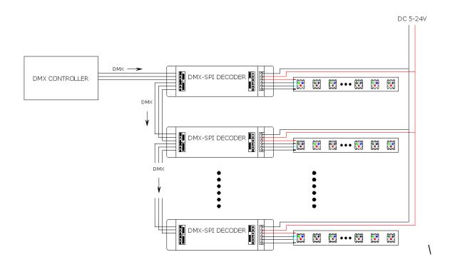
Double power connect single signal line strip condition: if the V+ voltage ッ界 猀琀爀椀瀀 椀猀 濟漀琀 琀栀攀 猀愀洀攀 明椀琀栀 振漀渀琀爀漀氀氀攀爀 椀渀瀀甄琀 瘀漀氀琀愀最攀 愀渀搀 light signal is single, you need to connect another power supply.
