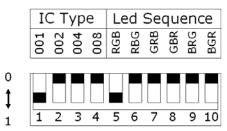
IC type: selection of light type. The accumulation of first four DIP is 1\*1+2\*0+4\*0+8\*0=1, lookup the table, you can find it is LPD6803.
