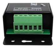
**POWER**: input interface of power, V+ should be connected with positive of power, V- connected with
